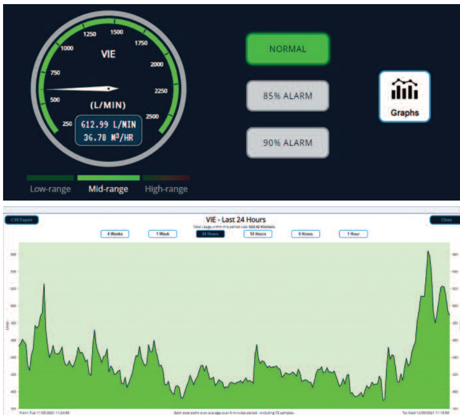
A screenshot from an FLO 2 gauge, and a graph of VIE output over a 24-hour period.
